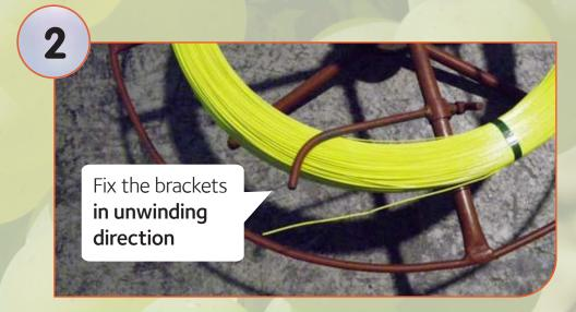
Cut the straps once the coil is well fixed
