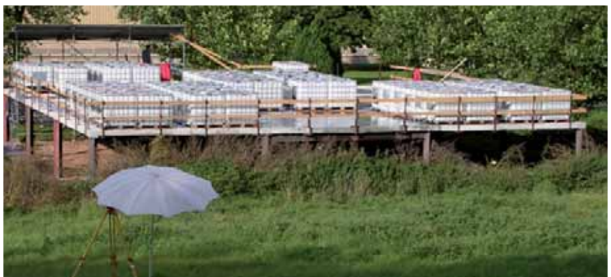
Figure 2: Checker board loading pattern of the Bissen test slab.
