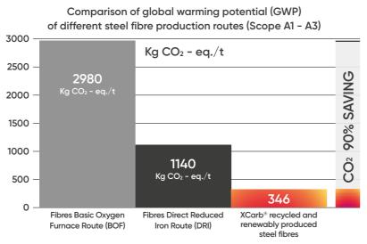
Kg CO<sub>2</sub> - eq./t values from EPD S-P-11903, EPD S-P-11871 and Steel Fibres Low Emission XCarb\* recycled and renewably produced EPD Self Assessment SA-11/23
