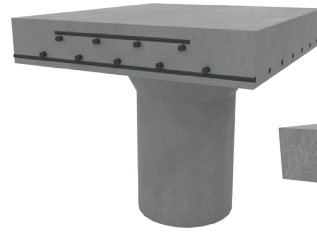
Slab on piles with traditional reinforcement
