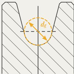
During a wire rope's lifetime, the rope diameter will decrease. This is due to first the elongation of the rope and then the wear on the rope wires. This diameter variation begins quickly but then slows down. The wire rope will create a new groove in the sheave which corresponds to the reduced diameter. If a new wire rope is installed in a worn sheave, without resurfacing, the new rope will wear more quickly. The lifetime can be divided by 10.
