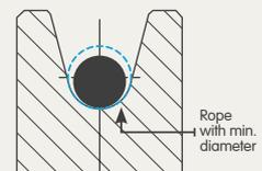
Wire rope after reduction diameter on correct groove
