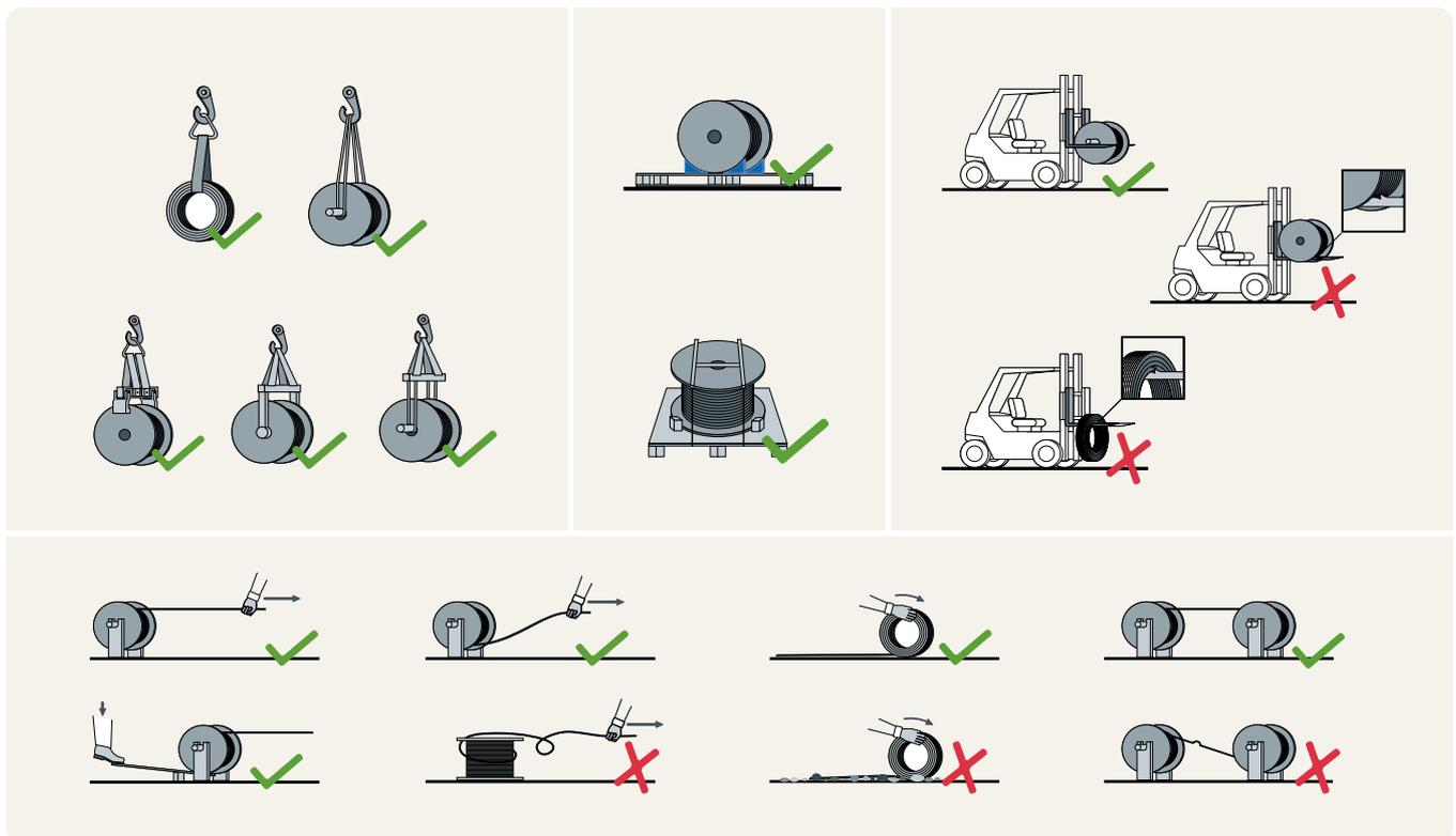
At all times, contact of the rope with any metallic pieces should be avoided to prevent early damage.
