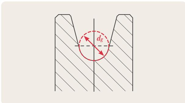
During a wire rope's lifetime, the rope diameter will decrease. This is due to first the elongation of the rope and then the wear on the rope wires. This diameter variation begins quickly but then slows down. The wire rope will create a new groove in the sheave which corresponds to the reduced diameter. If a new wire rope is installed in a worn sheave, without resurfacing, the new rope will wear more quickly. The lifetime can be divided by 10.
