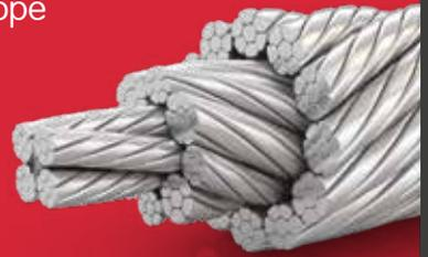
NRHD 24 is a rotation resistant rope for a broad spectrum of applications including tower cranes, mobile cranes, crawler cranes, high lift hoisting devices and deck cargo cranes. Excellent performance on multiple layer coiling winches along with a high resistance to bending fatigue.
