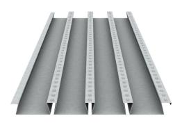
R51 is manufactured from S350 grade steel. This profile is a traditional re-entrant profile and is commonly used on inner city multi-storey projects where the structural zone and storey height is reduced, due to the relatively thin slab depth required to achieve a typical 1 hour fire rating.
