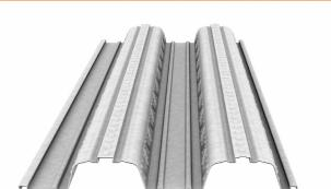
Initially added to our product range in 2002, the original TR80 has undergone further research and development, evolving to the now revised profile, renamed **TR80**<sup>th</sup>. This 80mm deep trapezoidal profile is available in 0.9mm, 1.0mm and 1.2mm gauges in both S350 and S450 grade steel.
