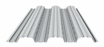
The TR60 profile was SMD's first trapezoidal profile, added to our product range in 1992. Further research and development in recent years has seen our trapezoidal products evolve into the TR+ range. The **TR60**<sup>⊕</sup> profile enables un-propped spans in excess of 3.5m and is available in 0.9mm, 1.0mm and 1.2mm gauges in both S350 and S450 grade steel.
