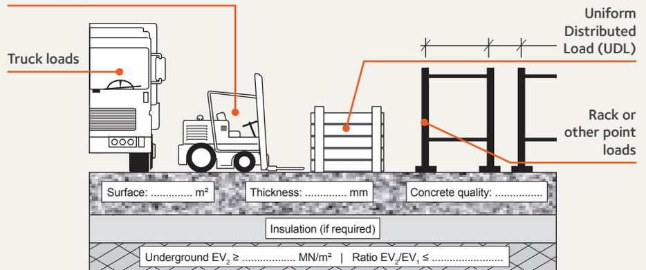
The design note will allow for the determination of the concrete grade, fibre type and fibre dosage rate. For certain loads it is extremely important to consider various aspects such as:
