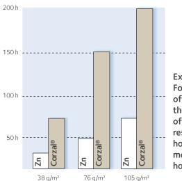
Example: For a coating of 105 g/m<sup>2</sup>, the duration of corrosion resistance is 72 hours for Zinc and more than 200 hours for Corzal<sup>®</sup>!
