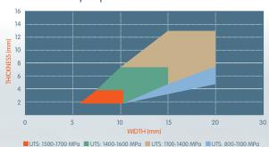
The chart above shows the mechanical properties according to the wire size.
