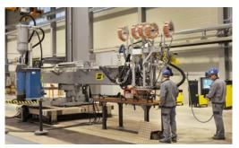
Welding laboratory: Multi-wire Submerged Arc Welding (SAW)
